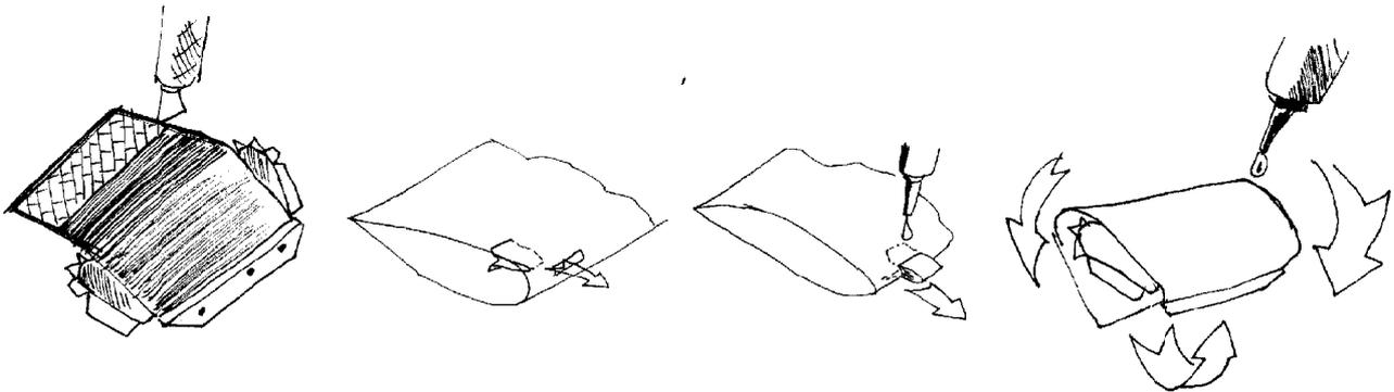
Cut the four elevons 5-10 & 5-11 and the body flap (5-8). Bend and fold them. Cut the hinges 5-9 for the elevons, 5-6 and 5-7 for the body flap. The 5-9, 5-6 and 5-7 have to pass through the slots and glued internally. Once dried, put the glue on the tabs and closes the elevons and flap.
