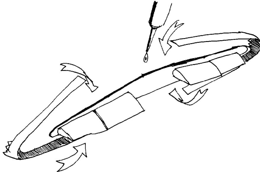
Cut and bend the 6-25 and 7-25. Glue the spar inside it as illustrated. The spar has to be aligned on the centerline. Glue the spar on the painted side, so that the unpainted side stay outside.
