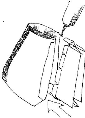
**Cut, bend and fold the vertical stabilizer 5-1. Insert the spar with rudders and close it with glue. Check that a large gluing tab has to protrude from the bottom part.**
