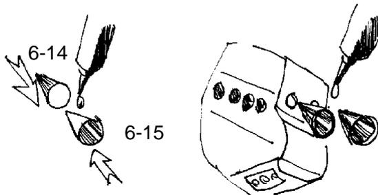
If you want you can cut the holes for the vernier thruster and insert the nozzles 6-16 and 7-16 inside the RCS part. 6-15 and 6-14 are mounted outside to form the two external nozzle of RCS
