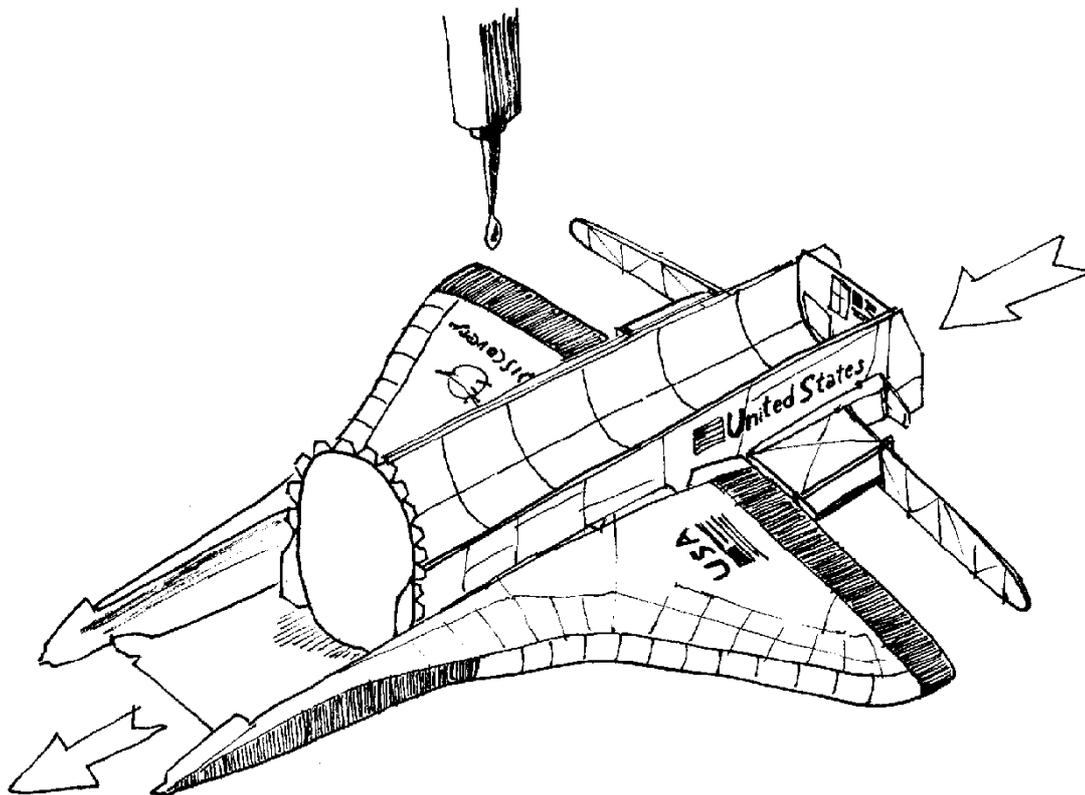
Try to bend both wings in the right shape by leaving weights on them during an entire night. Once the wing stay closed without weight, then insert the cargo bay sliding it from the back side. Glue the wings on the cargo bay tabs. Apply some glue also on the edges of the wing internal structure.
