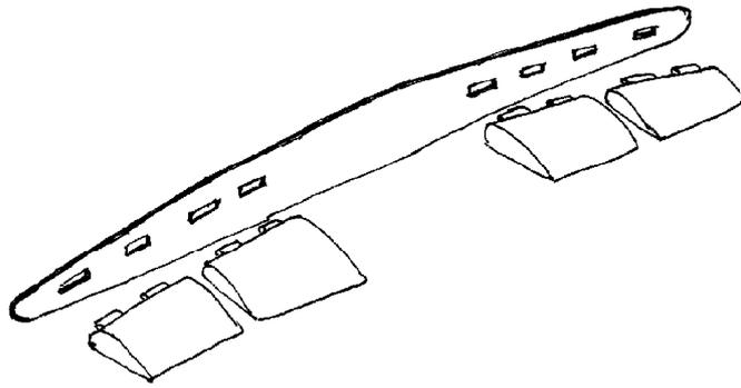
Insert the four elevant in the spar and glue them on the spar. You can also fix them to the spar by introducing a small paper roll inside the hinges once inserted into the slot
