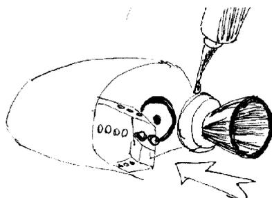
Mount the OMS right engine starting from the gimbal 6-20. Bend and glue it using the 6-22 and 6-23 tabs. Glue the 6-18 (external nozzle) and 6-19 (internal nozzle) together. Leave the hole at the center of the nozzle so that the injectors are visible through it. Glue the nozzle inside the gibal and then glue it to the OMS pod. Repeat the sequence for the left OMS pod.
