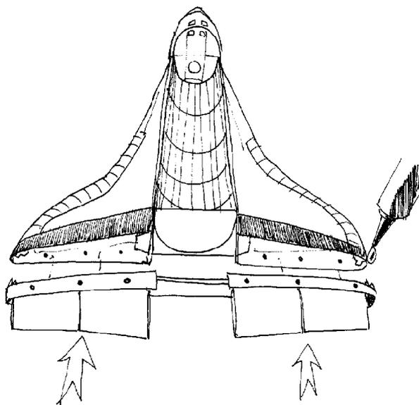
Once it is dried glue the part inside the wing. The spar has to be glued to the cargo-bay lower structure. The gluing tab at the tip are used to glue the black tip of the wings.
