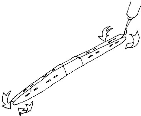
Cut the wings end spar 8-4, fold it and glue the two parts together. Cut the slots for the elevon hinges.
