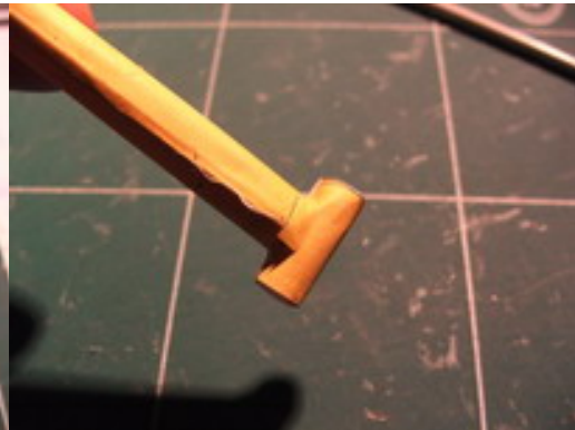
Glue items D and K to the outside of Items C and J after the glue has set as above.
