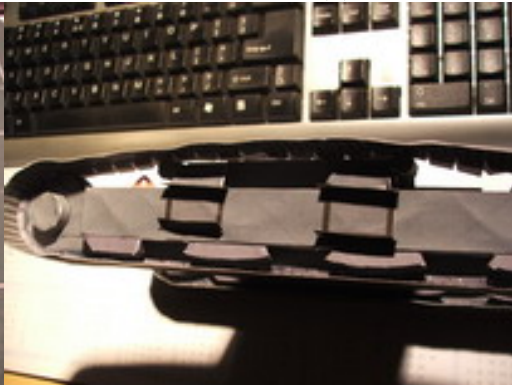
Glue items 165 to chassis as shown above on both sides,
