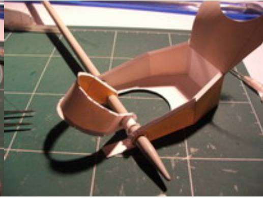
Glue the item 93, 96 assembly to item 94 as above, again use the 7.00mm needle as a guide.
