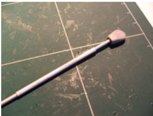
Cut and roll items 173 and 175 around a 2.0mm needle.
