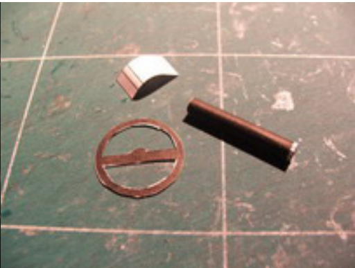
Cut fold, roll and glue items 203, 204 and 205 as above.
