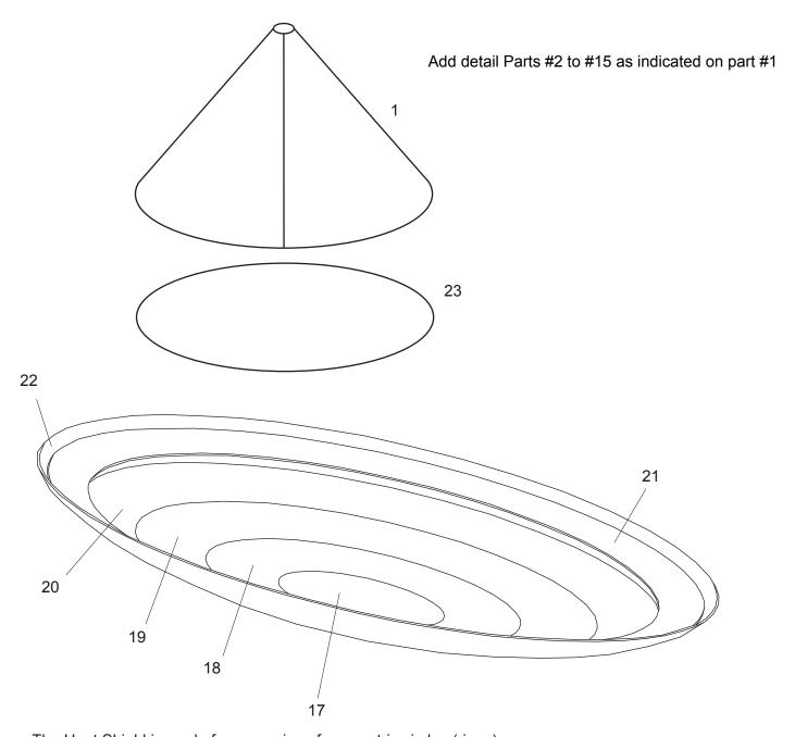
The Heat Shield is made from a series of concentric circles (rings).
