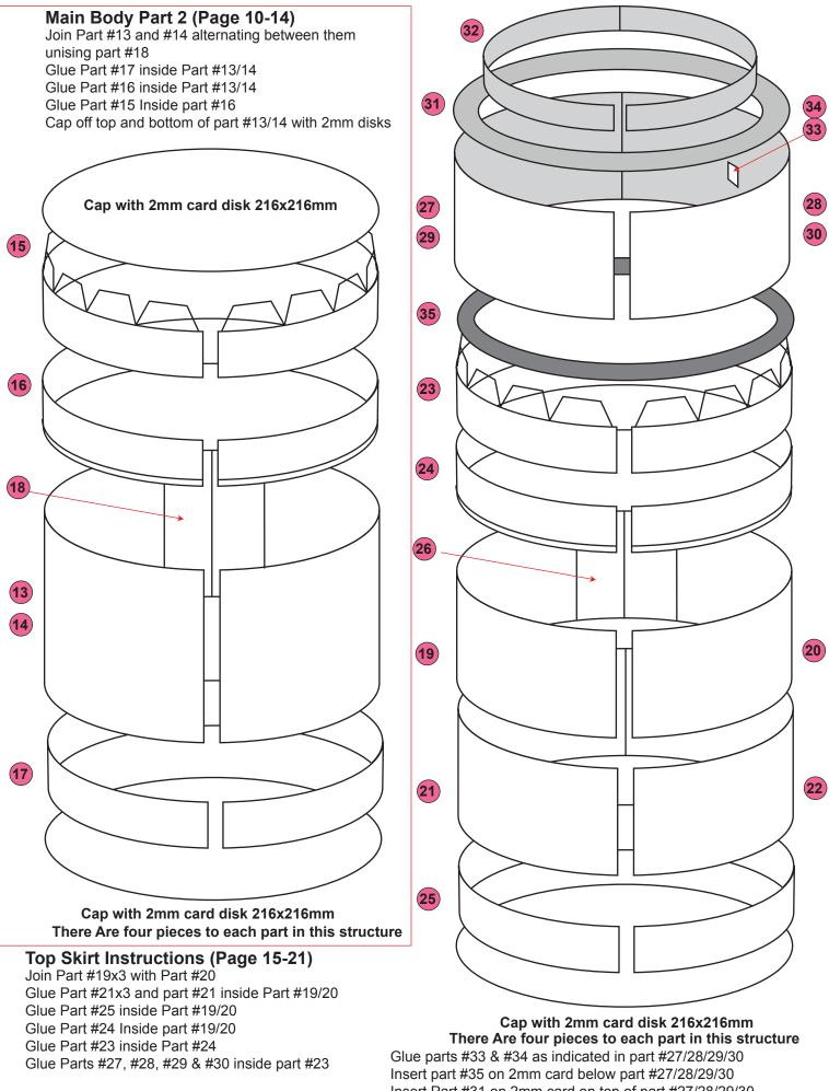
Insert part #35 on 2mm card below part #27/28/29/30 Insert Part #31 on 2mm card on top of part #27/28/29/30 after inserting dome then insert part #32 inside part #31 inner ring Cap off base of part #19/20 with a 2mm card disk
