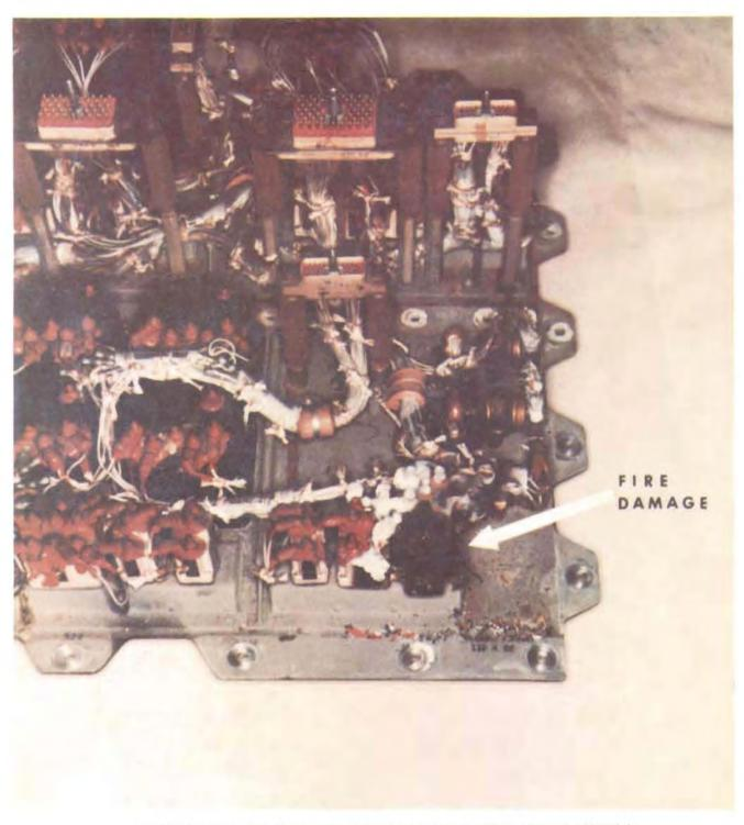
INTERIOR VIEW OF PANEL 13 SHOWING DAMAGE NEAR THUMB WHEELS
